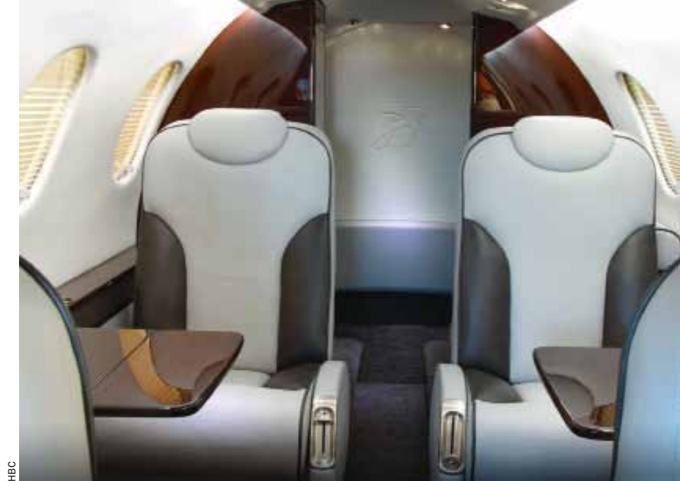
Each club seat has pitch, recline, lateral track and swivel adjustments, plus a retractable aisle-side armrest.
