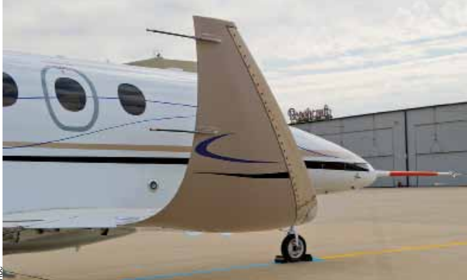
The Hawker 200's elliptical winglets, developed in partnership with Wichita-based Winglet Technology LLC, are the most obvious aerodynamic change to the aircraft from its predecessor.
